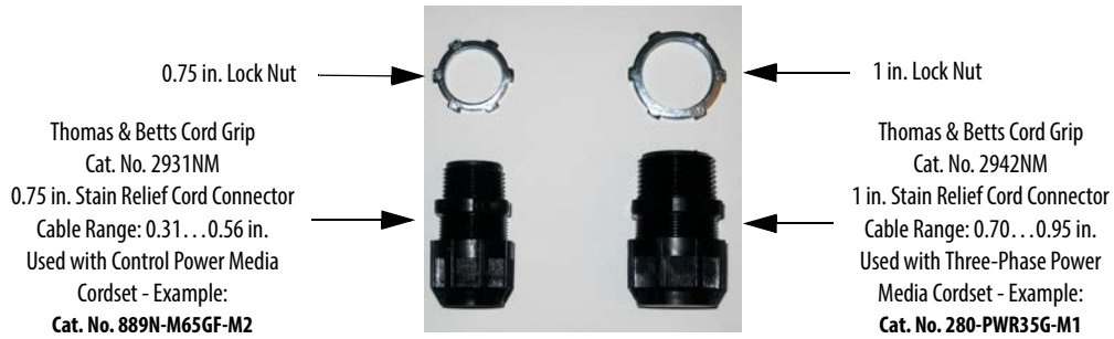
Figure 34 - Cord Grips for ArmorStart Devices with 25 A Short Circuit Protection Rating
