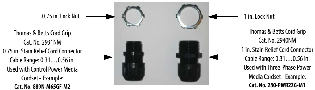
Figure 33 - Cord Grips for ArmorStart Devices with 10 A Short Circuit Protection Rating
